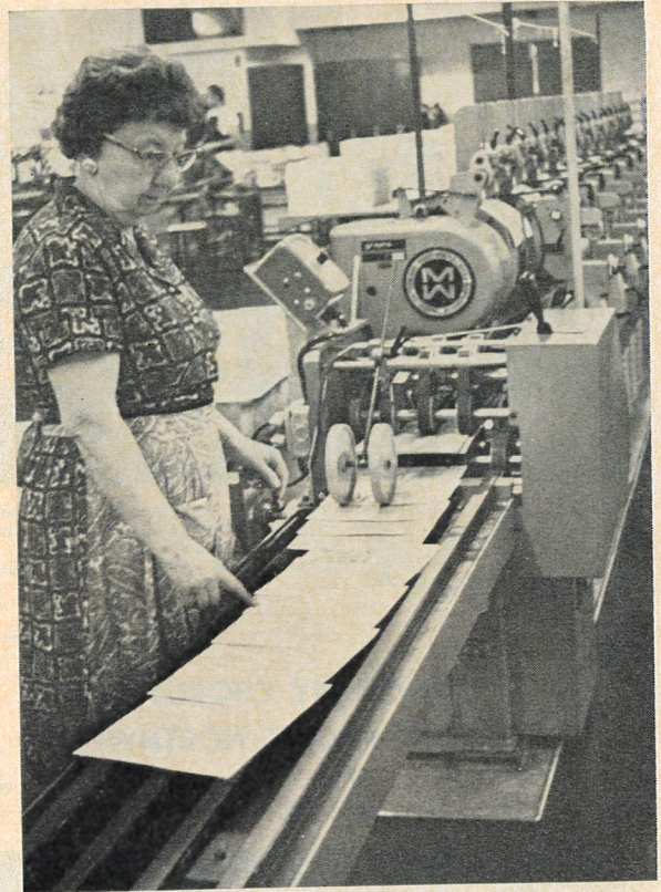
A collator, pictured here, gathers either the sections of a book or the sheets of loose-leaf items, such as Seat Work and Home Study Work in Sunday-school materials or Catechism Study Exercises.
