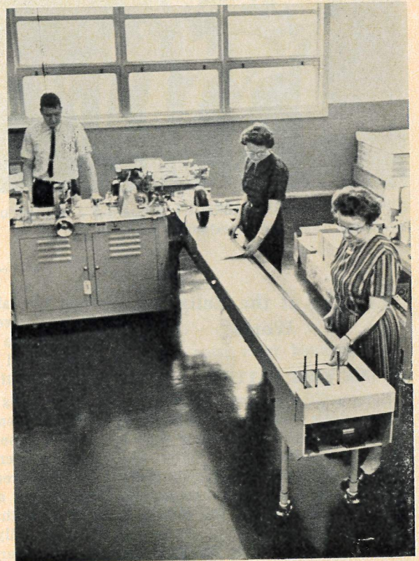
In the Mailing Department one finds the labeling machine. Your Northwestern Lutherans are rolling off the belt. It attaches the mailing labels to the copies. It can handle 20,000 units per hour.
